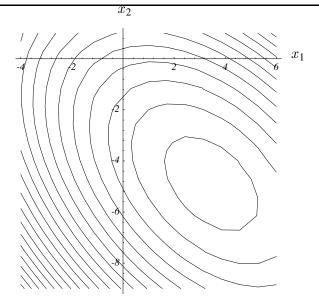
Figure 36: Contour lines of the quadratic form of the diagonally preconditioned sample problem.
