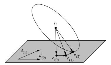
Figure 26: In this figure, the shaded area is  $e_{(0)} + \mathcal{D}_2 = e_{(0)} + \operatorname{span}\{d_{(0)}, d_{(1)}\}$ . The ellipsoid is a contour on which the energy norm is constant. After two steps, Conjugate Directions finds  $e_{(2)}$ , the point on  $e_{(0)} + \mathcal{D}_2$  that minimizes  $\|e\|_A$ .
