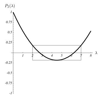
Figure 33: The polynomial  $P_2(\lambda)$  that minimizes Equation 50 for  $\lambda_{min}=2$  and  $\lambda_{max}=7$  in the general case. This curve is a scaled version of the Chebyshev polynomial of degree 2. The energy norm of the error term after two iterations is no greater than 0.183 times its initial value. Compare with Figure 31(c), where it is known that there are only two eigenvalues.
