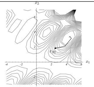
Figure 41: The preconditioned nonlinear Conjugate Gradient Method, using the Polak-Ribière formula and a diagonal preconditioner. The space has been "stretched" to show the improvement in circularity of the contour lines around the minimum.
