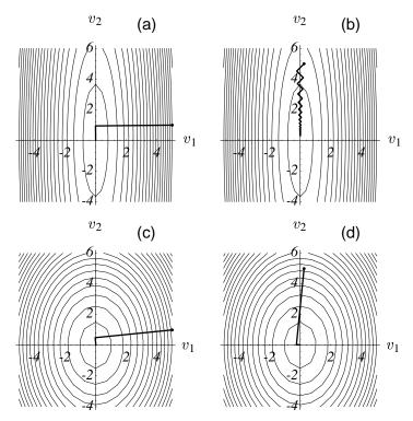
Figure 18: These four examples represent points near the corresponding four corners of the graph in Figure 17. (a) Large  $\kappa$ , small  $\mu$ . (b) An example of poor convergence.  $\kappa$  and  $\mu$  are both large. (c) Small  $\kappa$  and  $\mu$ . (d) Small  $\kappa$ , large  $\mu$ .
