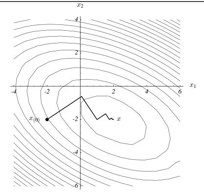
Figure 8: Here, the method of Steepest Descent starts at  $[-2, -2]^T$  and converges at  $[2, -2]^T$ .
