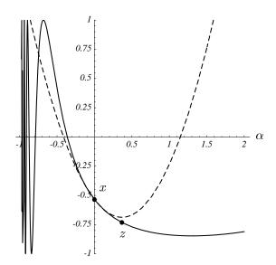
Figure 39: The Newton-Raphson method for minimizing a one-dimensional function (solid curve). Starting from the point x, calculate the first and second derivatives, and use them to construct a quadratic approximation to the function (dashed curve). A new point z is chosen at the base of the parabola. This procedure is iterated until convergence is reached.
