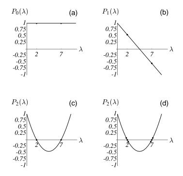
Figure 31: The convergence of CG after i iterations depends on how close a polynomial  $P_i$  of degree i can be to zero on each eigenvalue, given the constraint that  $P_i(0) = 1$ .
