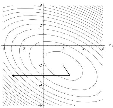
Figure 25: The method of Conjugate Directions using the axial unit vectors, also known as Gaussian elimination.
