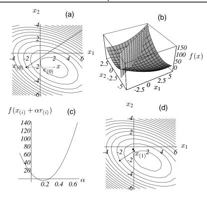
Figure 6: The method of Steepest Descent. (a) Starting at  $[-2, -2]^T$ , take a step in the direction of steepest descent of f. (b) Find the point on the intersection of these two surfaces that minimizes f. (c) This parabola is the intersection of surfaces. The bottommost point is our target. (d) The gradient at the bottommost point is orthogonal to the gradient of the previous step.
