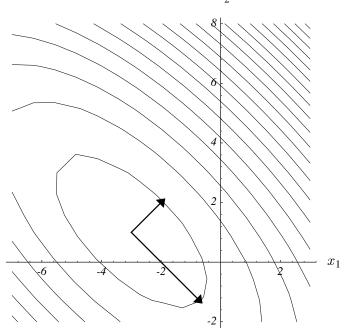
Figure 16: The energy norm of these two vectors is equal.
