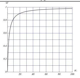
Figure 20: Convergence of Steepest Descent (per iteration) worsens as the condition number of the matrix increases.
