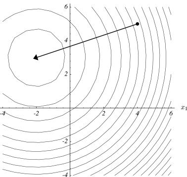
Figure 15: Steepest Descent converges to the exact solution on the first iteration if the eigenvalues are all equal.
